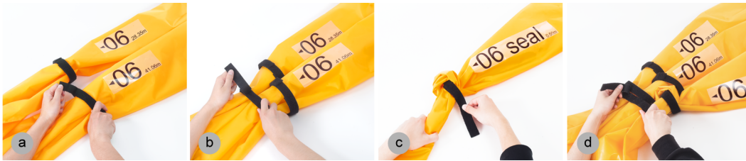
Figure 15: (a-b) We construct regular, airflow-permitting nodes using Velcro ties. Adding (c-d) forming a loop and then feeding a Velcro strip through blocks airflow at nodes next to the actuators.
