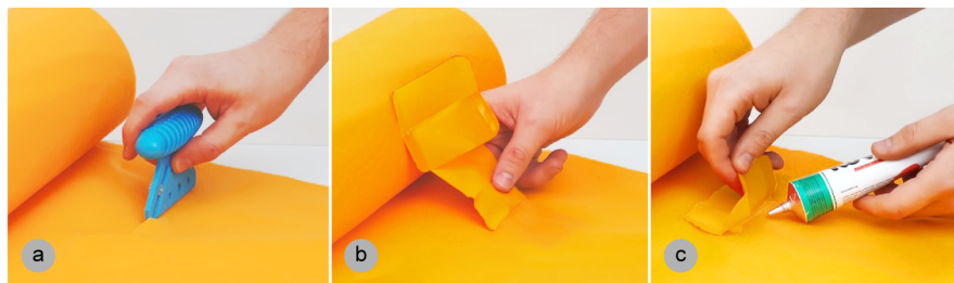
Figure 11: Users mount a custom inlet by (a) cutting, (b) inserting, and (c) gluing.
