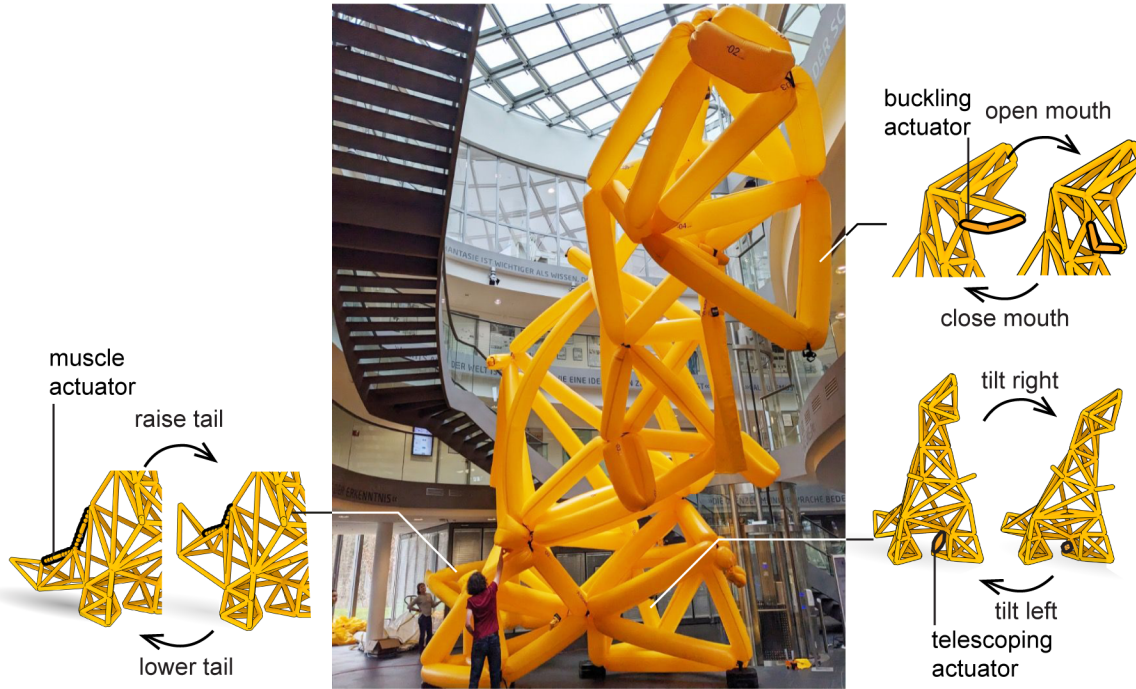
Figure 2: 16m long and 8m high animatronics sculpture of a T-Rex, made from 250m tube.
